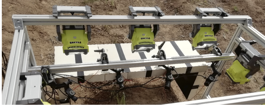
Figure 3.6: Early Version of Vision System Hardware Setup. The proposed system contains 3 cameras and 4 lights inside a darkened enclosure.
