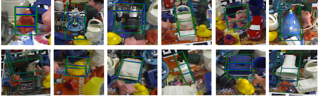
Figure 5.5: Visualisation of qualitative results on the LINEMOD dataset. Green bounding boxes represent ground truth poses and blue boxes represent the refined poses.
